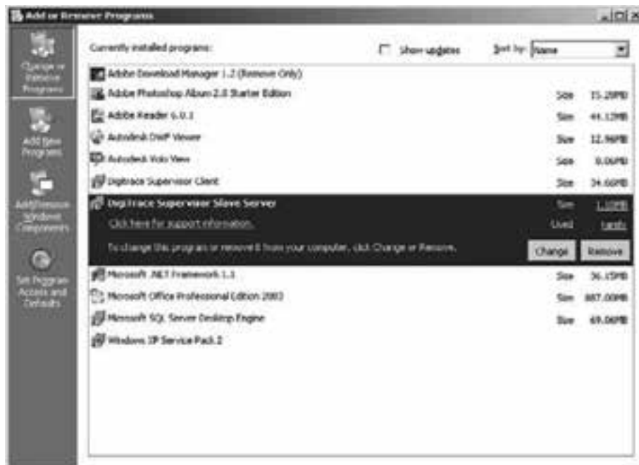
Figure 3-46 Remove DTS slave server
